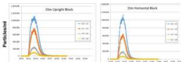
Fig. 8. Effect of 1/8" tubing orientation. 15m upright block: rise: 02:20; decay: 03:22. 15m horizontal block: rise: 02:12; decay: 03:57. Loss of peak intensity is 5% to 50%, worse for larger particles.
